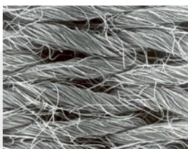
ACTIVATED CARBON FILTER (ACF)
