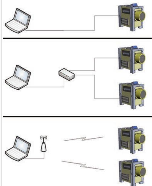
Detective-Remote measurement solutions are easily configured to meet the CONOPS requirement that USB and wireless communications methods be provided.
