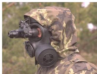
The lenses of the OM-90 mask were computer designed to ensure compatibility with all kinds of optical devices while providing a sufficient field of vision.
