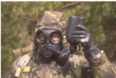
The OM-90 mask is equipped with a drinking device which enables safe drinking from a special plastic bottle (PE, 0,8 l) in a contaminated area.
