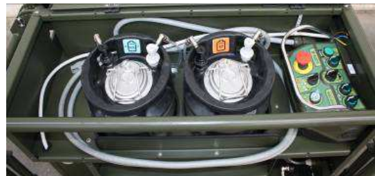
Pressurized containers for XP PREMIER and hydrogen peroxide
