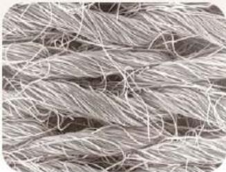
Filter material made of knitted activated carbon fibers, laminated on both sides with a polyamide comfort liner.
